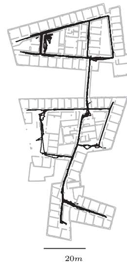
Fig. 6. Combined trace of robot location over all deployments
